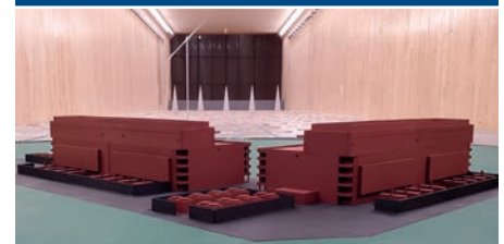
Simulating exhaust dispersion in the wind tunnel ensures that all relevant building features are included.
