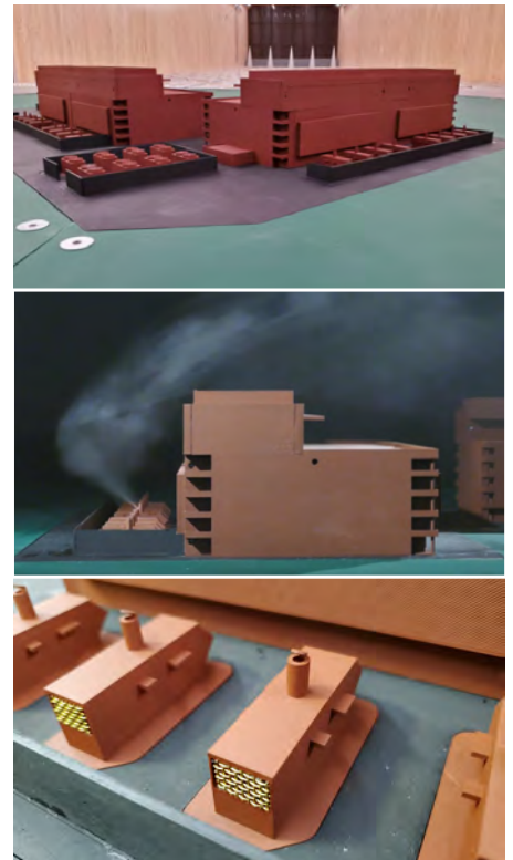
Hyperscale data center in the wind tunnel - the model is placed on a turntable, so all possible wind directions can be evaluated.
