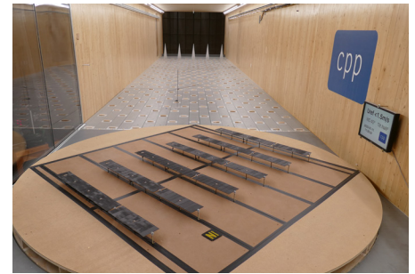
3D aeroelastic studies predict wind-induced instability and help identify stowing procedures to prevent catastrophic damage.
