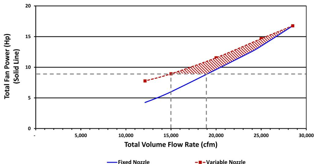
Figure 6. Fan curves of volume flow rate vs. fan power for a fixed-nozzle stack and a variable-nozzle stack that maintains a constant exit velocity.
