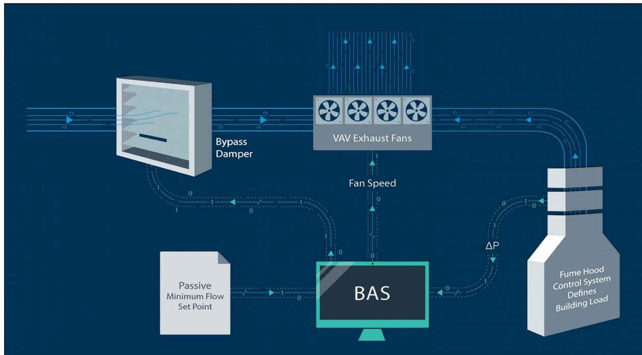
Figure 7. Simple turndown VAV control strategy flow diagram.
