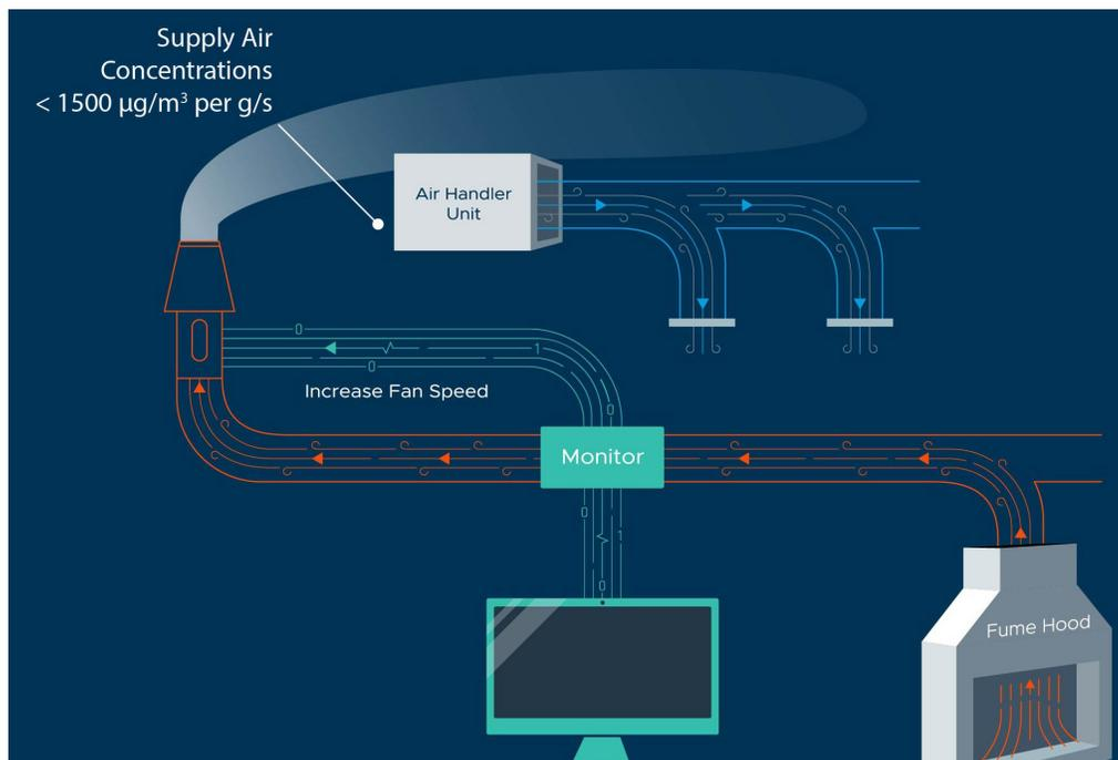
Figure 9. Lower plume rise and higher intake concentrations are allowable when measured concentrations within the exhaust stream are below the monitored threshold value. (Note this does not necessarily mean the exhaust stream is “clean” of any contaminants, just that they are not detectable.)
