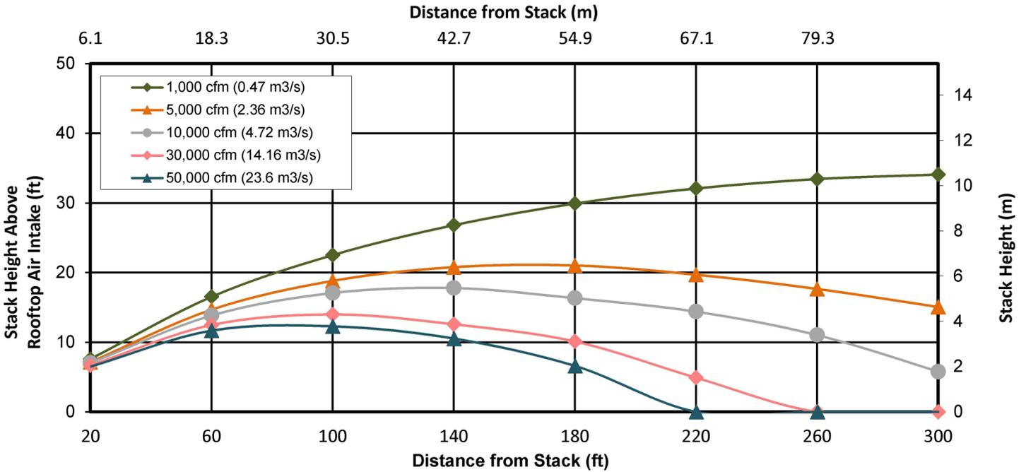
Figure 4. Stack height above top of intake required to meet a specified design criterion for various exhaust volume flow rates at a range of downwind distances. (Design criterion =  $400 \mu\text{g}/\text{m}^3$  per g/s;  $V_e = 3,000 \text{ fpm}$  [ $15.2 \text{ m/s}$ ].)
