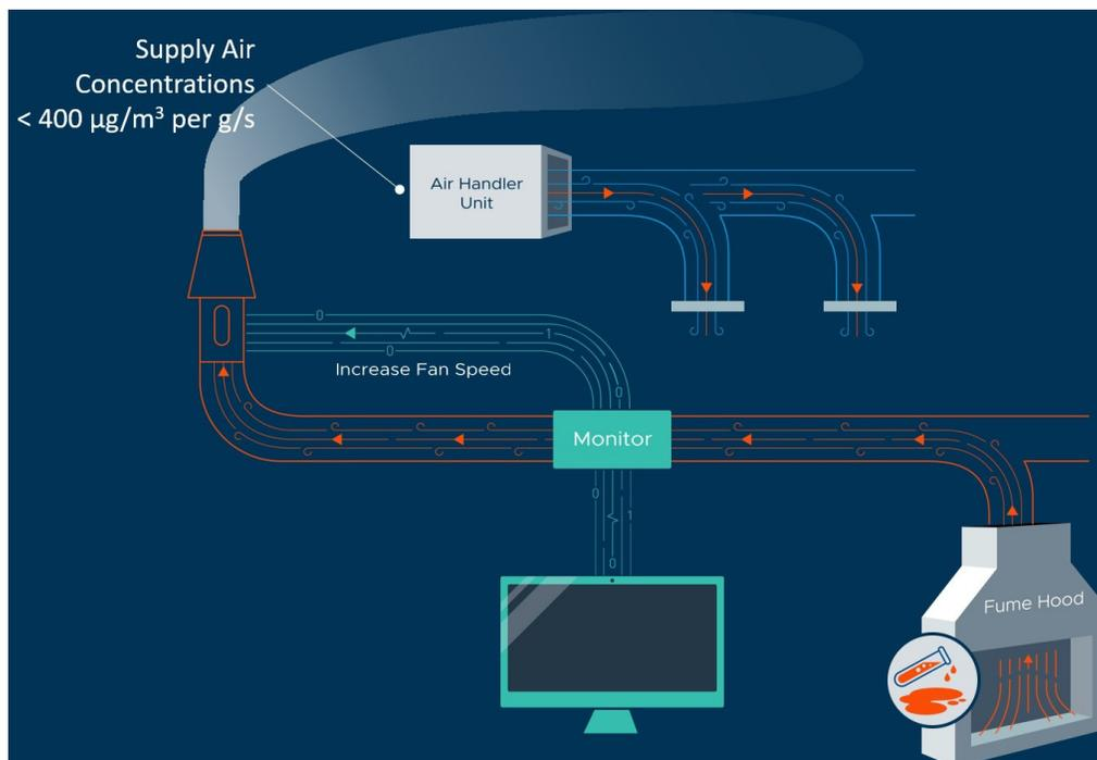
Figure 10. When chemical concentrations in the exhaust stream are above the monitored threshold value, the exhaust volume flow rate is increased, creating greater plume rise and reducing downwind intake concentrations.
