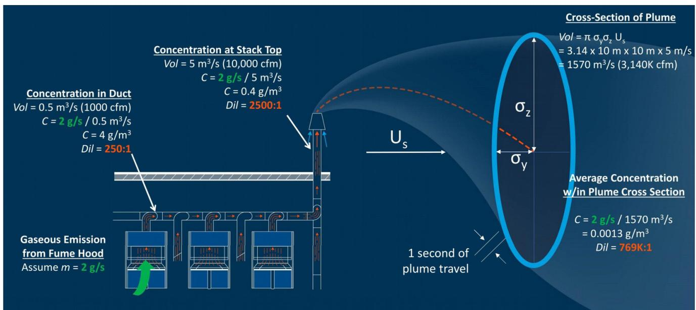
Figure 3. Example of concentration distributions downwind of an induced-flow fan, illustrating that the induced flow has no impact on downwind concentrations.
