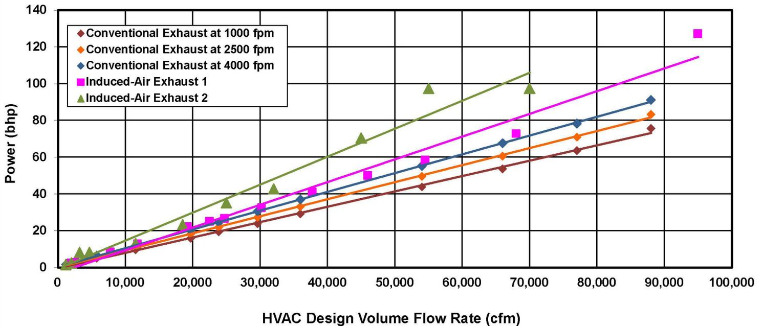
Figure 5. Required fan power vs. HVAC design exhaust volume flow rate (at 4-in. w.g.).
