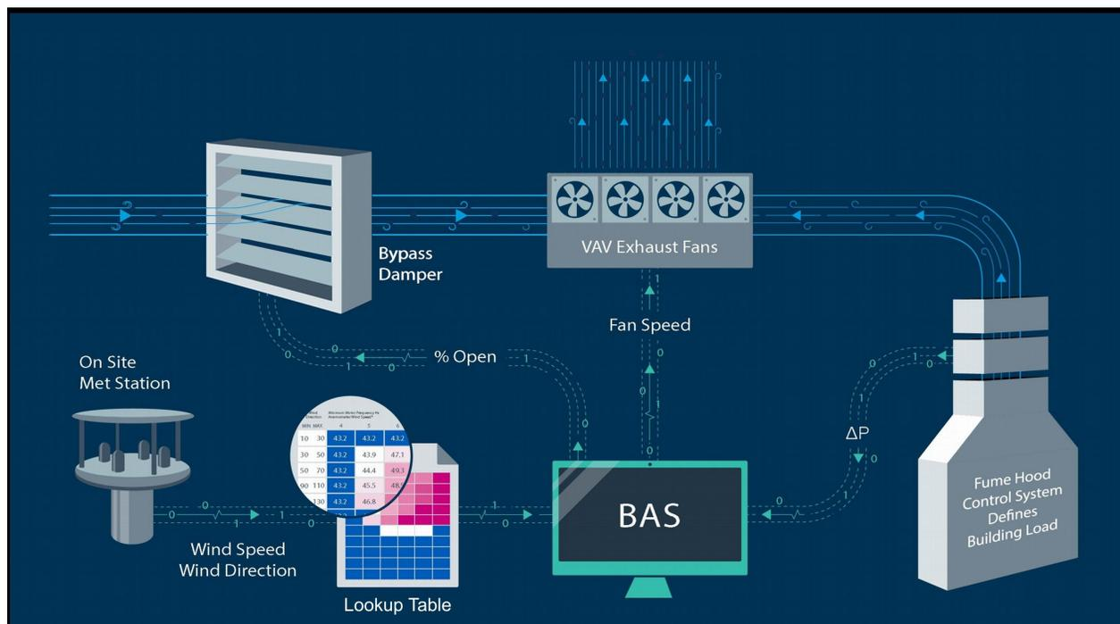
Figure 8. Wind-responsive VAV control strategy flow diagram.
