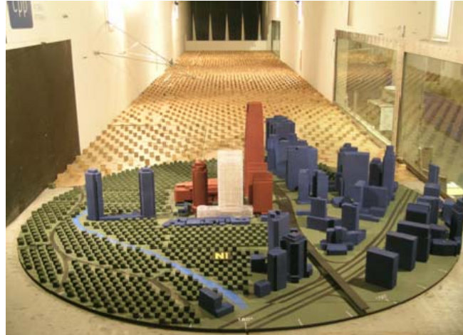
Figure 1: Wind tunnel model of Jakarta City Centre in one of CPP's boundary-layer wind tunnels.
