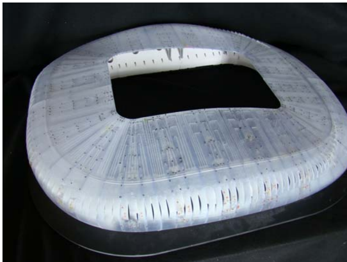
Figure 8: Hundreds of simultaneous pressure tap pairs used on the roof of the Monterrey Stadium in Mexico.
