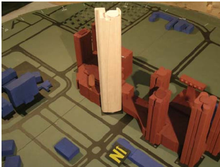
Figure 4: Base balance testing of the St Moritz Tower in Jakarta.
