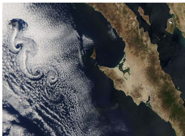
Figure 5: Naturally occurring Von Kármán vortex shedding downstream from island
