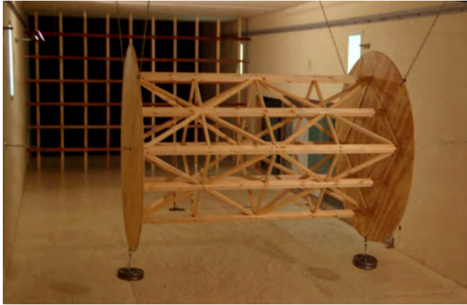
Figure 6. A simple static section-model test of extended spire cross-section type BB (8 columns).
