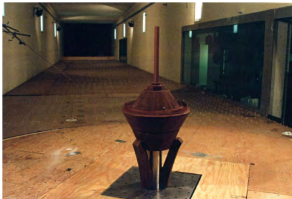
Figure 10. Enlarged 1:150 model used to study flow patterns and speeds in the area of the observation deck.
