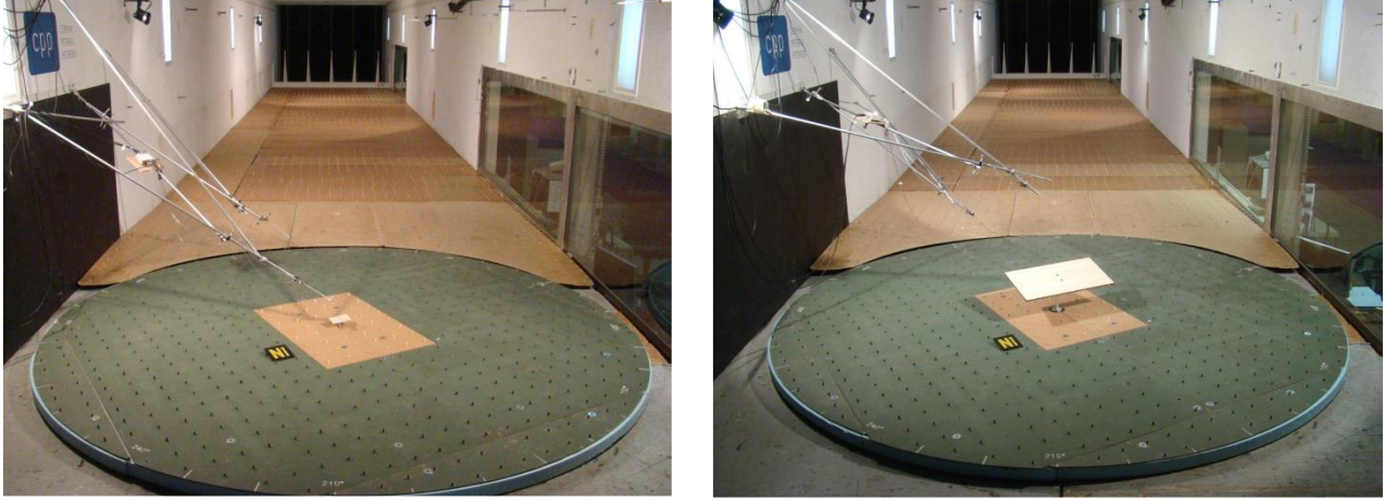
Figure 1. Boundary layer wind tunnel tests at scales (a) 1:50 and (b) 1:250
