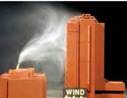
Exhaust being drawn upwind
