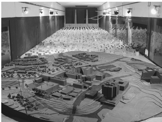
Figure 9 Photograph of a model installed in an atmospheric boundary-layer wind tunnel.
