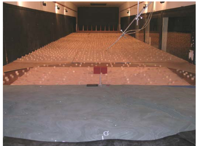
Figure 4. Photograph of wind tunnel configuration for EBD testing
