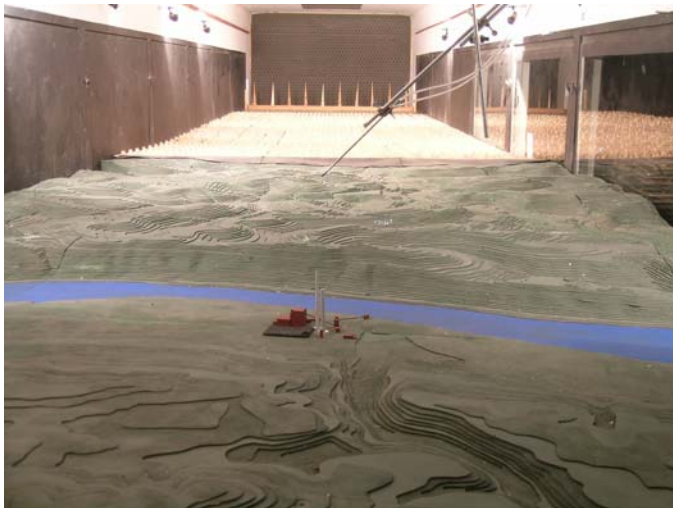
Figure 3. Photograph of wind tunnel configuration with terrain present
