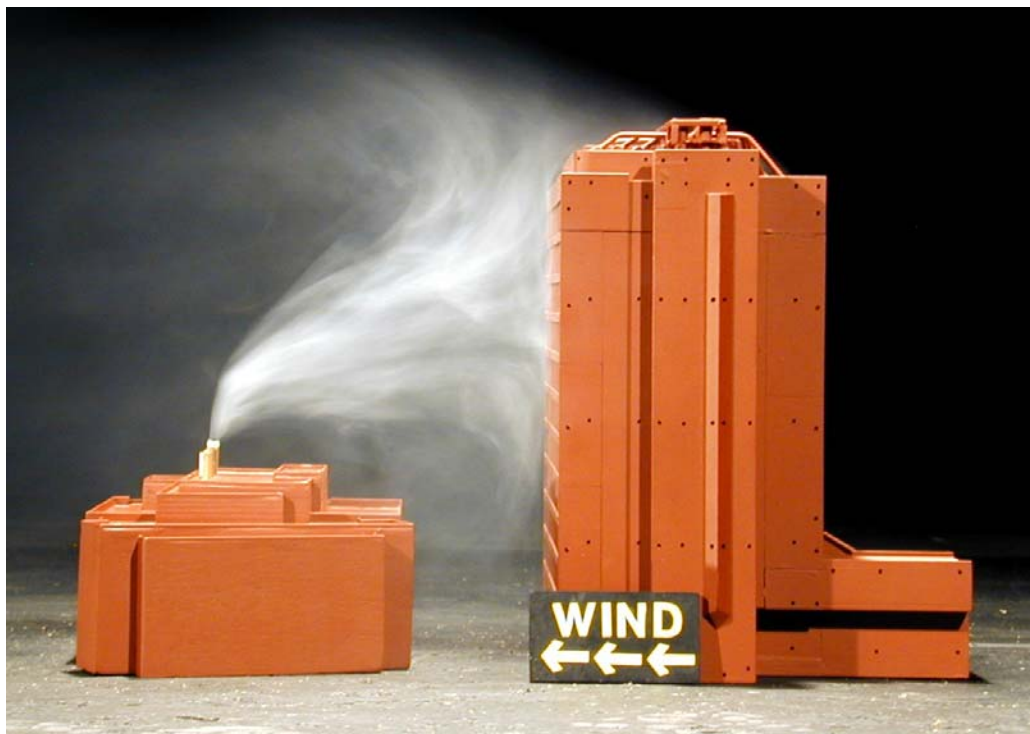
Figure 7 - Plume caught in taller, upwind building cavity.
