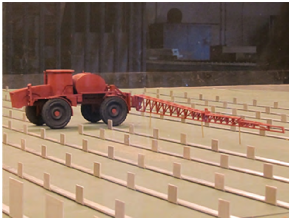
Figure 1. (top) Layout of the tunnel looking upwind with the spray rig rotated 45° to the wind and (bottom) side view of the scale model at 0° to the wind. The locations of the roughness elements are adjusted depending on wind direction and the desired probe measurement locations.
