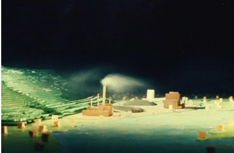
Figure 12: wind tunnel model of downwash behind a ridge.
